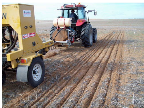
Figure 2 (LEFT): Andrew Bird (SANTFA) driving the tractor towing the FLOW 55,000psi injector in front of the Serafin Ulti-sow disc-seeder at Karoonda.
