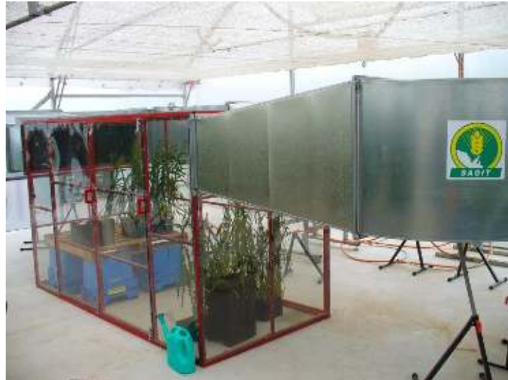
Figure 3 The heat chamber developed for the current project to produce relevant, controllable and repeatable conditions to screen for heat stress response in plants.
