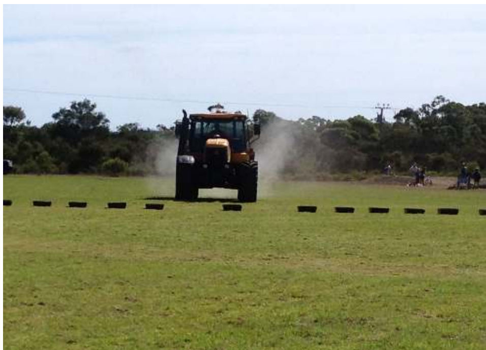
The Southern Spreader on a JCB truck driving across the collecting trays
