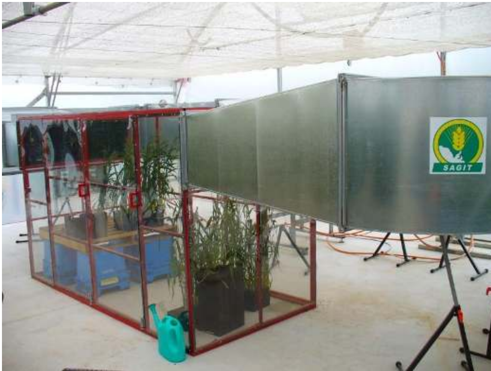
Figure 1: The heat chamber developed for previous bread wheat projects with AGT and SAGIT, and which was used for the current project to produce relevant, controllable and repeatable conditions to screen for heat stress response in durum germplasm.
