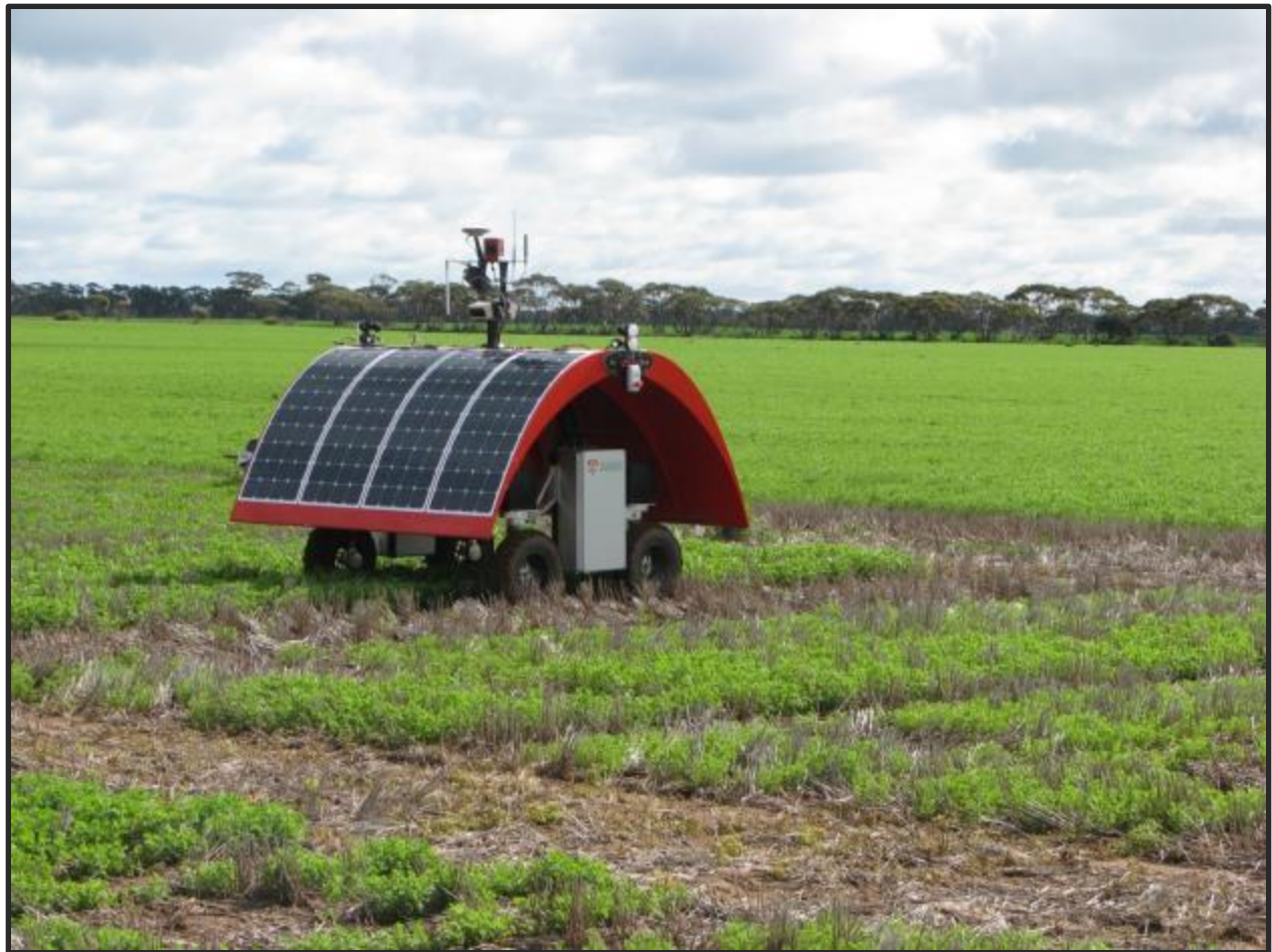
The Ladybird robot (ACFR) in action autonomously imaging lentil plots at Pinery
