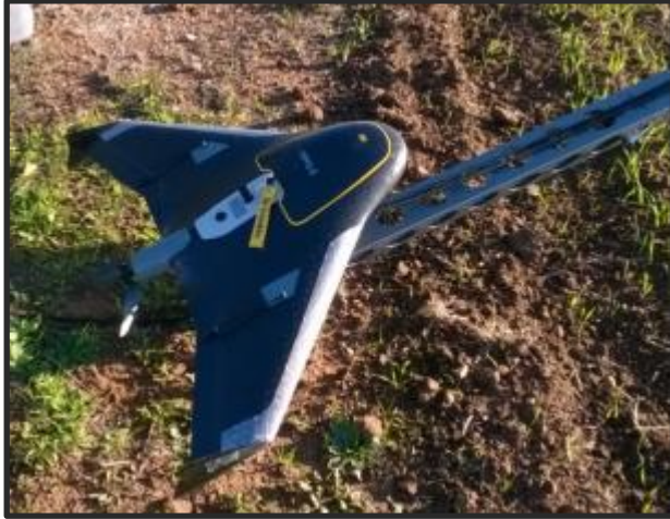
Close-up of the Trimble UX5 used for my research
