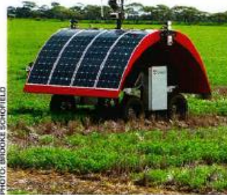
A SARDI research project tested how autonomous and aerial devices could be incorporated into field trials. They used the prototype Ladybird robot (left) and a UAV (right).
