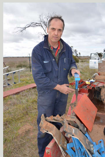
Dr Jack Desbiolles with a bent leg opener at the Moorlands trial site
