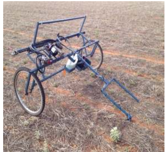
Figure 5. Plot sprayer (2m; 12 volt motor) used to apply broad-acre herbicides.
