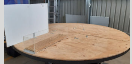
Above: Grain testing container on the ship motion simulator.
