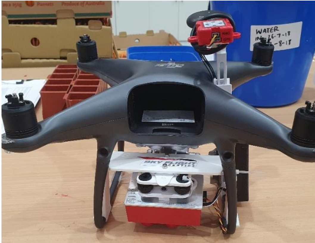
Figure 4: Phantom 4 Pro with MicaSense Red Edge Camera Integrated
