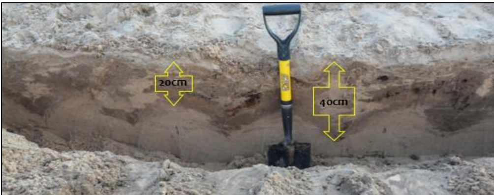
Photo 5. Indication of Spading pattern on Sand (approx. 40cm depth)
