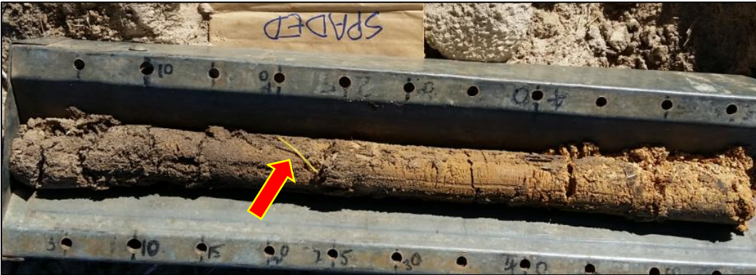
Photo 5. Indication of Spading pattern on Sand (approx. 40cm depth)
