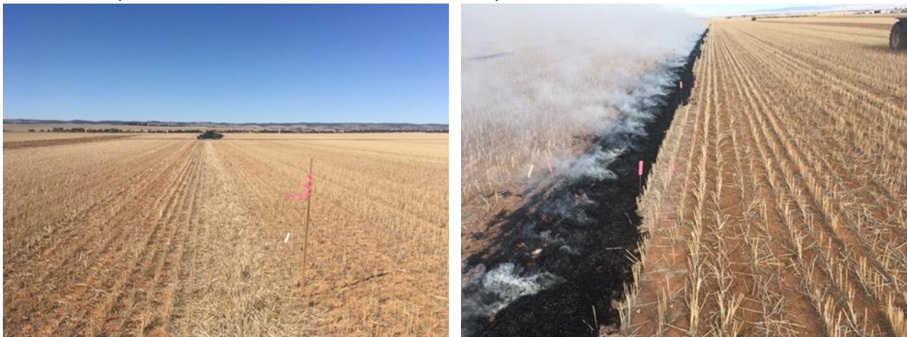
The pre-emptive flame retardants showed capacity to inhibit the spread of lesser fires away from windrows.
