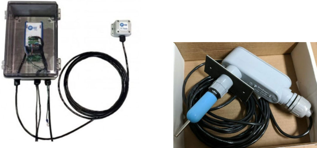
Figure 42. Fan control node (left) and fan plenum sensor (right)
