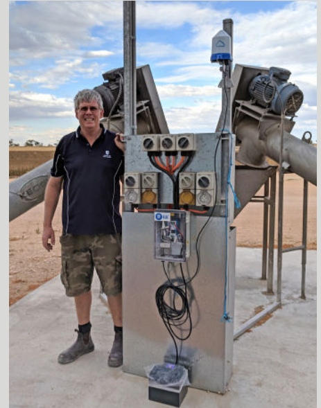
Professor John Fielke with an OPI cable data system used to monitor silo conditions.
